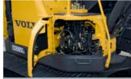
• Wide open, ground level service area provides easy hydraulic valve access.
