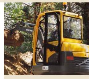
Open door is protected in the width of the chassis.
