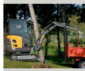
· Protected, smartly-positioned boom cylinder.
