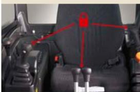
Controls lock when the safety strut is raised.
