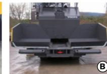
A high transport speed of 6 km/h and extraordinary manoeuvrability facilitate moving the paver around the jobsite. Individually operated hopper wings (option) and swivelling truck buffer rollers permit paving right up to lateral obstructions.
